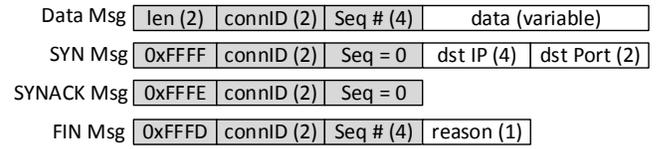
**Figure 3: Pipe message format with headers (8 bytes) shaded.**
