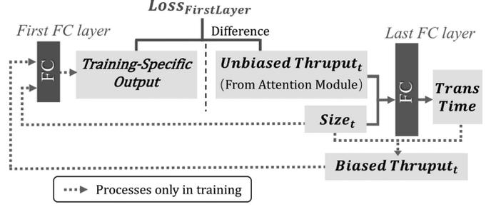
Fig. 8. The second part of the loss function we set in the TTP model training (i.e.,  $Loss_{FirstLayer}$ ). The output of the first FC layer is a training-specific output for self-supervised bias transformation learning.
