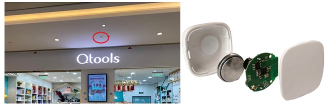
Figure 1: BLE Beacon on ceiling.
