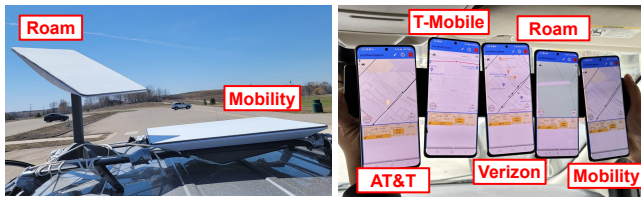
Figure 2: Two dishes are mounted on the rooftop and five smartphones are placed side by side in the vehicle.
