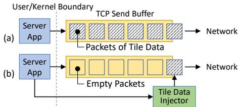
**Figure 8: Two server-side transmission schemes.** Flare uses (b).
