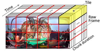
Figure 1: Chunk, tile, frame, and tile segmentation (4×6 tiles).
