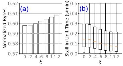
**Figure 15:** Impact of  $\xi$  on (a) downloaded bytes and (b) stall time (simulation).
