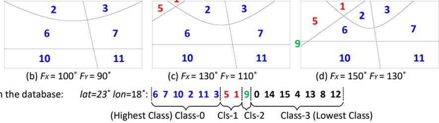
Figure 7: Ranking the tiles and deriving classes for a viewport. Assume 4x4 tiles and 4 classes.
