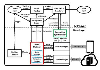
Figure 3: System architecture of CARS framework (dotted lines are for control messages). Its two key components are Scene Matcher and Annotation Synchronizer.
