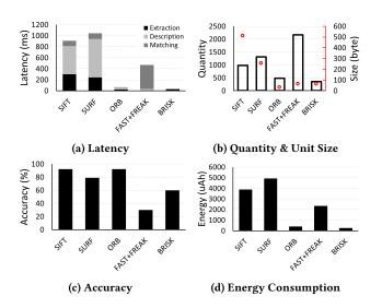
Figure 5: Performance comparison of various algorithms using OpenCV4Android library on a Xiaomi MI5 phone.
