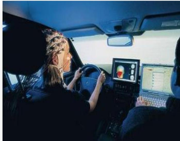
**An EEG Based Assistant Driving System Developed by DaimlerChrysler Company**
